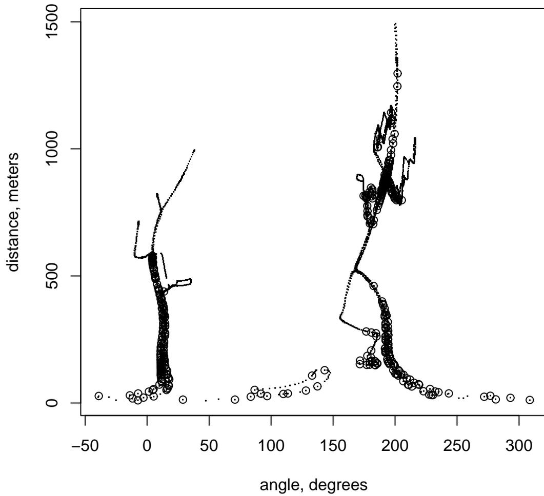
FIGURE 9: Angle versus distance for recorded points. Circles are points with positive through-put. Angle has been rotated such that zero is approximately east, and 180 is approximately west (inverted when compared to the map in figure 8).
