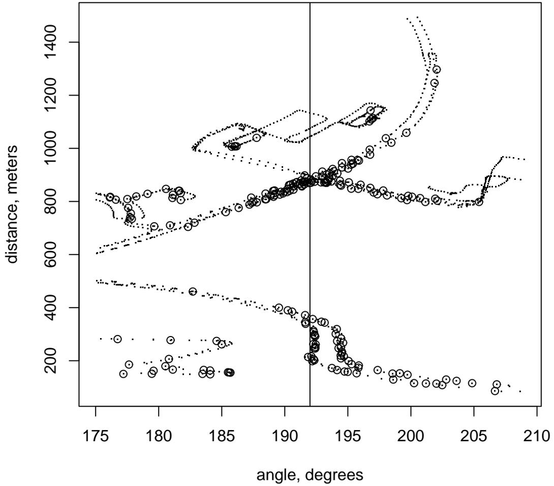
FIGURE 10: Angle versus distance for recorded points, for a 34 degree band around 192 degrees. Circles are points with positive throughput.
